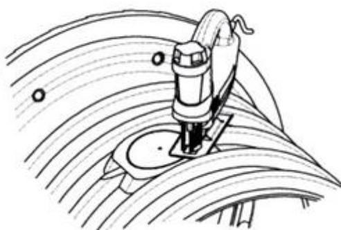
The connection areas have circular saw markings, the diameter of each is appropriate for the use of lamella gaskets DN 100 or DN 125, see 1.1. The sawing can be done with an appropriate hole saw or a jigsaw (see figure).
